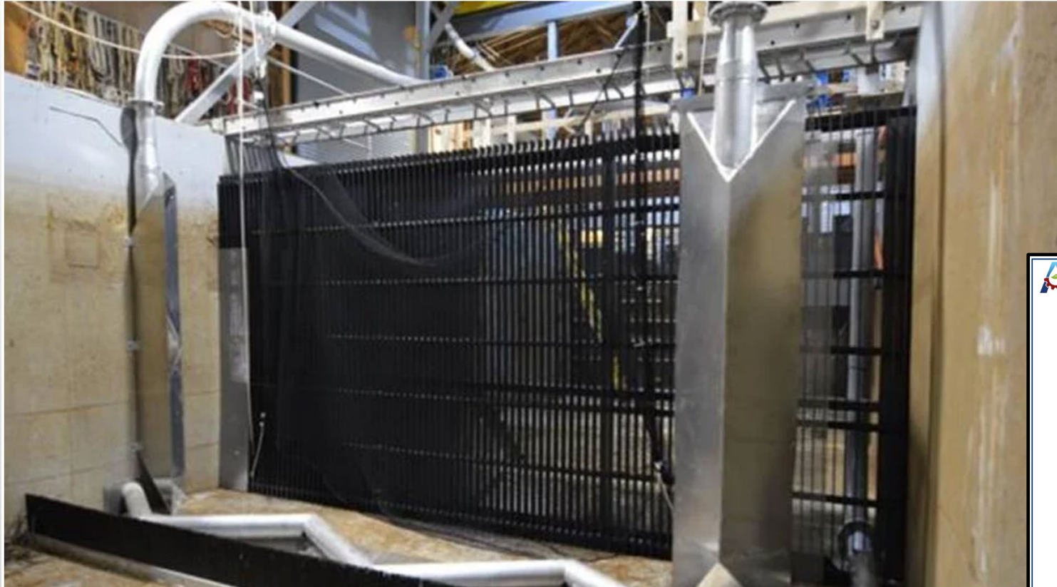
The laboratory evaluation was conducted in a large re-circulating flume using the Klawa horizontal zig-zag eel bypass system and a vertical eel bypass system developed by Lakeside Engineering
