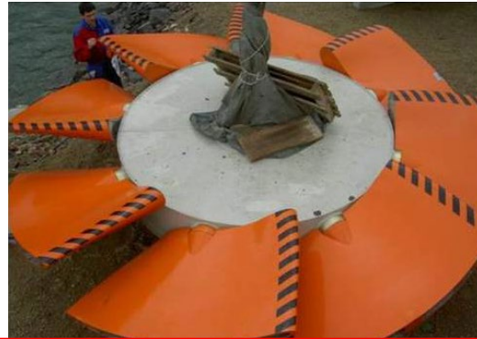
MJ2 Technologies Very Low Head turbine (VLH) < 12 ft head
