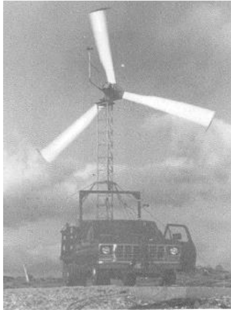
Figure 53 Typical Operation in Wind Speeds Below 11 m/s (Good Alignment)
